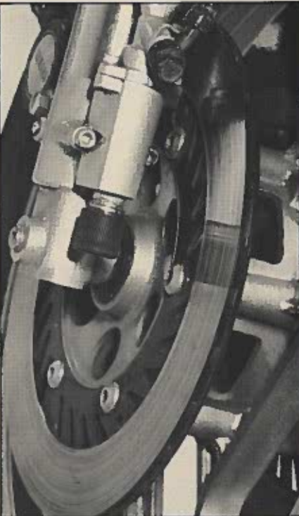
Knobs on fork legs set anti-dive; the ventilated discs need surprisingly high lever effort.
