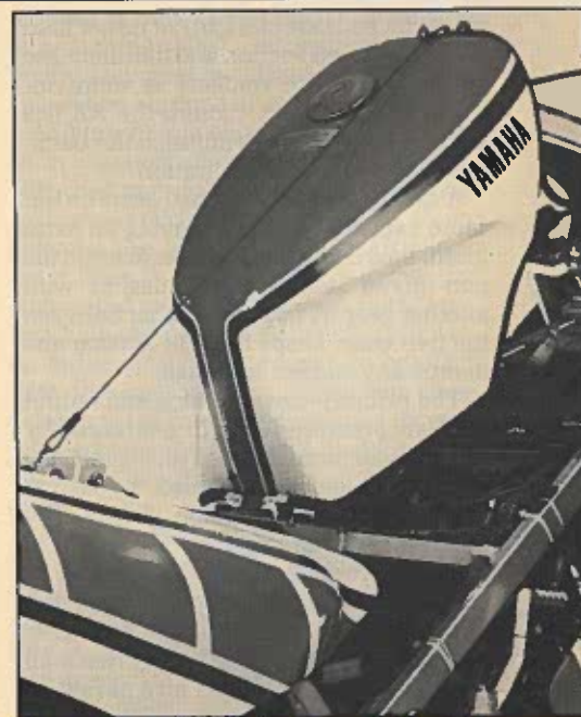
The air filter and rear cylinders can be reached by tilting back the hinged tank.
