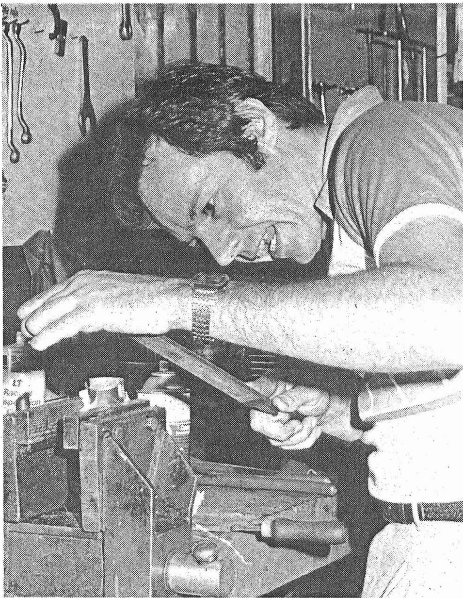
Rob Assink fine tuning the carby slide cutaway using the old flat bastard....
