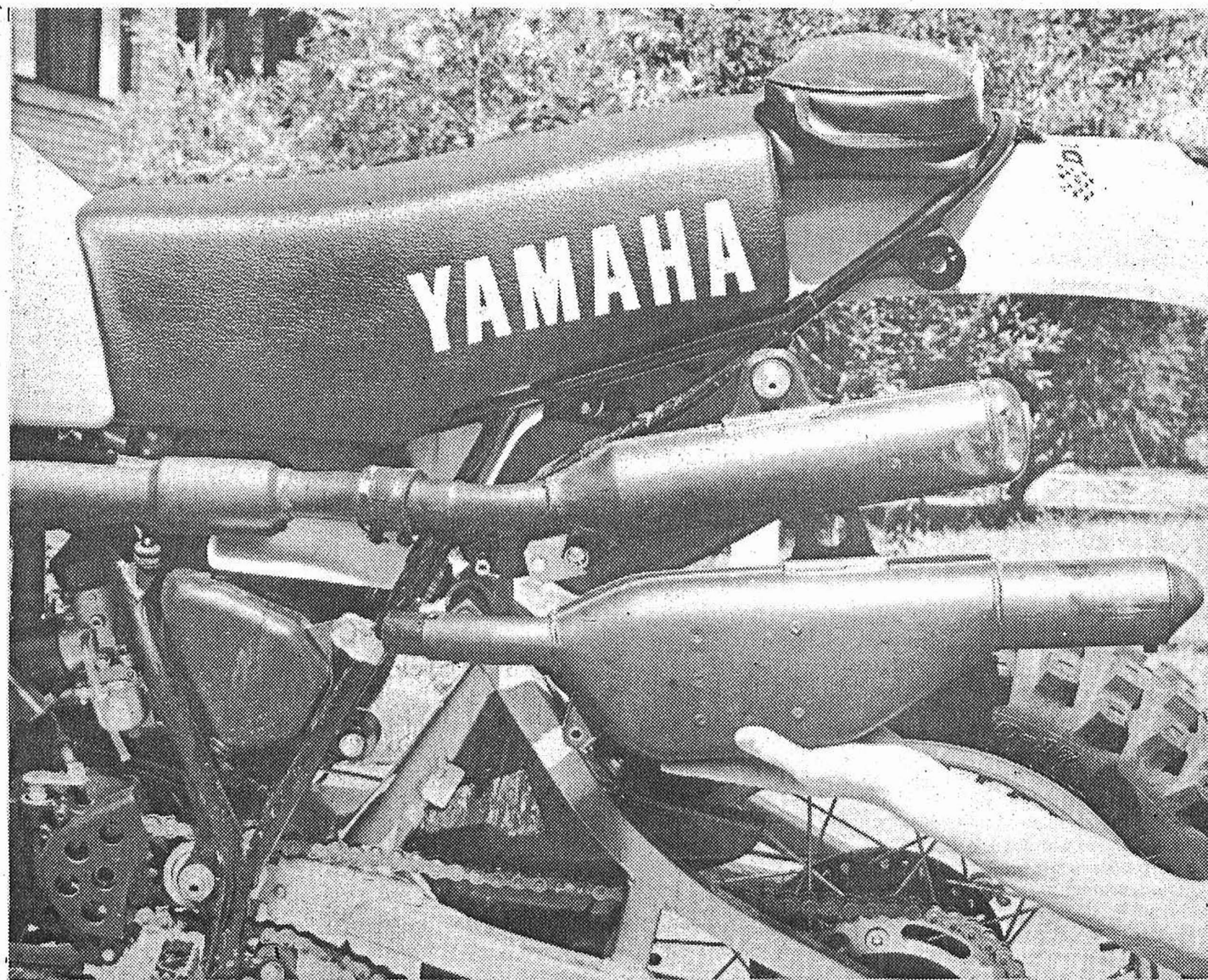
Above: the bulky and restrictive standard muffler dwarfs the YZ465H replacement.
