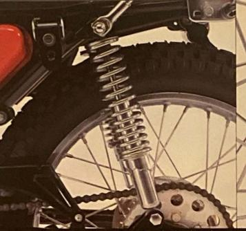
Adjustable rear shocks can be set to the load you're carrying or the condition of the road. Yamaha's dust and water resistant brakes have traditionally set the industry standard for sure stopping
