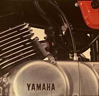
Torque Induction, Yamaha's unique intake system, utilizes a reed valve to feed the engine the exact amount of fuel and air it needs. The result is that horsepower is increased, particularly at low rpm's.
