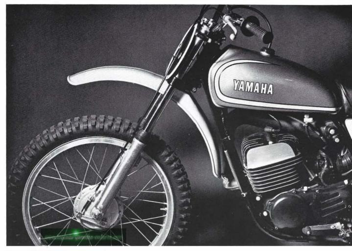
One of the first things that strikes the eye is the new, lower engine placement and the new up-and-across expansion chamber.
