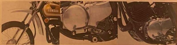
New high-clearance fender of lightweight polypropylene is virtually unbreakable. New front fork design and new steering geometry help 1974 Yamaha Trails handle like motocrossers on rough trails. Constant-mesh five-speed transmission has short throw selector for quick, smooth shifts. Yamaha gearboxes are notoriously rusped.
