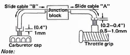
To measure the amount of cable slack, slide the cable back and forth over the throttle wire, and see how much end gap exists between the cable end and top of the carburetor (or cable guide 'A', if checking throttle cable 'A' slack).
