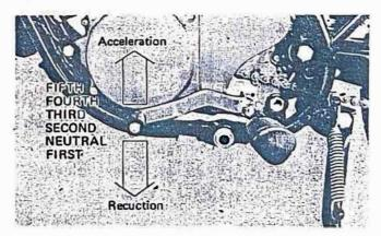
To shift into NEUTRAL, depress the change pedal to the end of its travel (you will feel a stop when you are in low gear), then raise it slightly.
