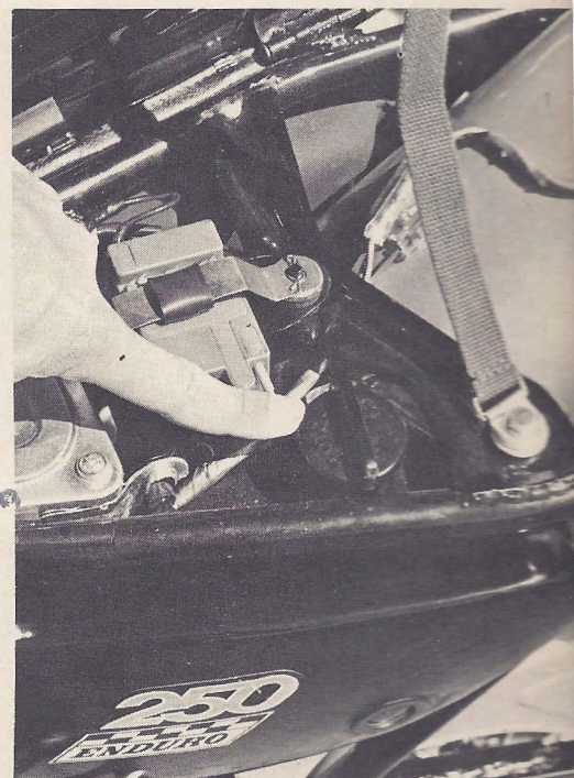
Air cleaner, battery and oil tank filler cap are all under the seat. A quick-disconnect for the tail light is behind the oil tank.
