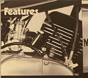
Torque Induction, Yamaha's unique reed-valve intake system, feeds the engine the exact mixture of fuel and air it needs. The result is more horsepower, particularly at low rpm's. Autolube monitors engine load and speed then automatically mixes oil and fuel accordingly. Constant flow adjustment to meet operating conditions helps extend engine life.
