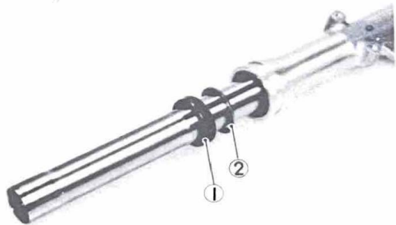
1. Oil seal 2. Oil seal washer
