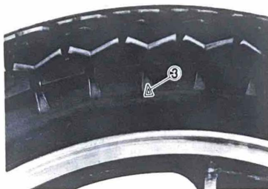
1. Tread depth 2. Side wall 3. Wear indicator
