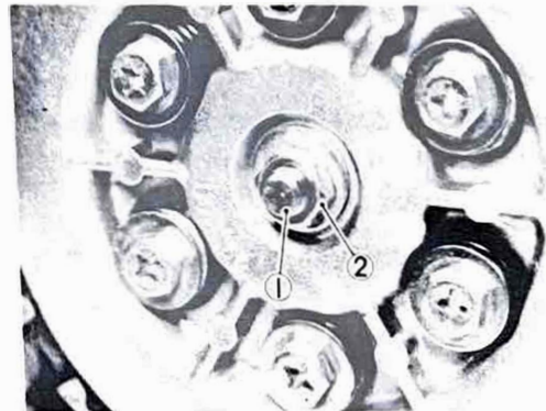
1. Adjusting screw 2. Locknut
