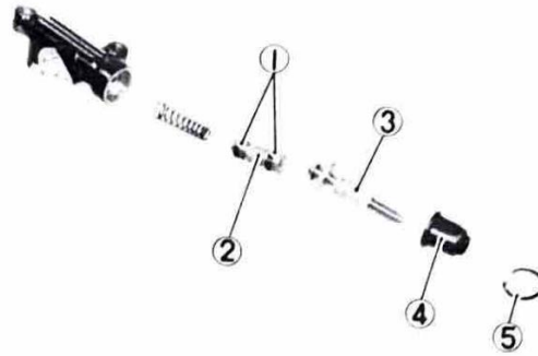
1. Cup 2. Piston 3. Snap ring 4. Dust boot
