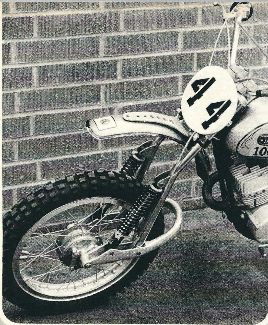
The Swenco leading link fork assembly and Koni shock combo does wonders for handling on fast, rough terrain.
