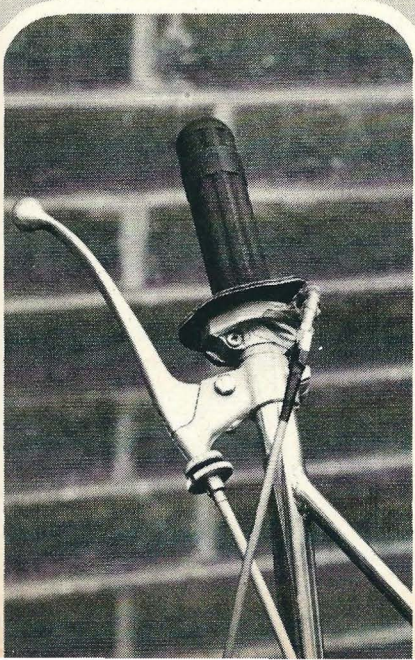
The attention to small details on any bike can contribute to winning ways. Here soft grips and leather hand protectors keep the rider from getting fatigued.
