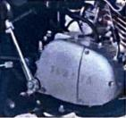
Smooth is the word for the 5-speed transmission. Gear changes are quick and effortless. Note also that primary kick starter permits starts in any gear
