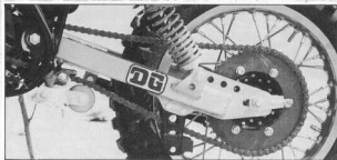
Along with the new swingarm and shocks, DG gave the Kawi a new chain guide and tensioning system to direct the bigger drive system.
