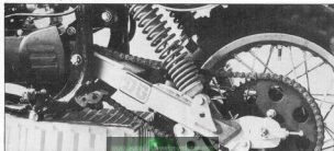
Reservoir KYB shocks add an inch-plus to the rear travel, and the new chain and gearing give the bike a better, stronger pull.
