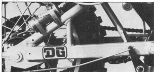
A new swingarm and Luft shock add travel to the YZ's rear.
