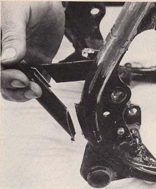
21 Cut off the bottom of the bracing tube as close to the frame member as possible. Leave the bracing ear in place.
