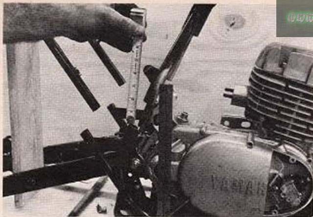
9 With the down tubes set at two inches, set the main rear tube at the same vertical measurement. With the down tubes parallel the rear, tubes will be close on.
