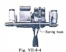
In actual practice, there will rarely be need to adjust the cutout relay. If the point surfaces of the voltage and cutout relays are worn or pit
