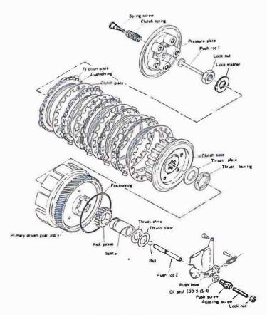
Fig. IV-9-2 Clutch ass'y exploded view
