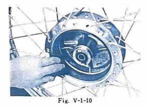
Check the spokes. If they are loose or bent, replace or tighten
