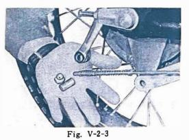
Loosen the chain tension adjusting nuts and bolts on both right and left sides.
