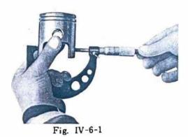
To determine the maximum piston diameter, measure the piston with a micrometer at right angles to the skirt 10 mm. (3/8 in.) from its bottom edge. (Fig. IV-6-1)
