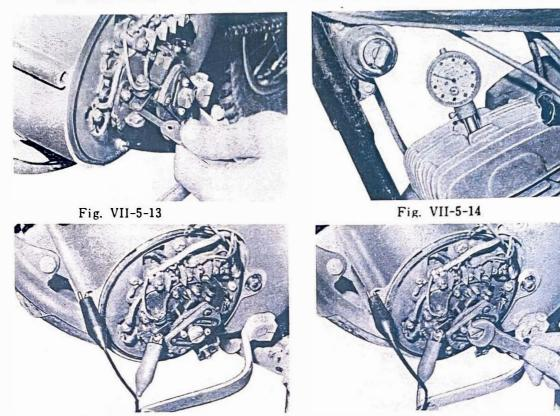
and then bring the piston up to exactly 1.8 mm B.T.D.C. (Fig. VII-5-16).
