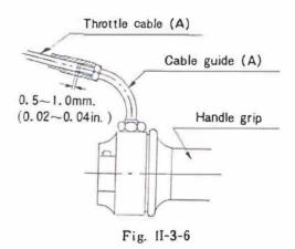
• Check the play of the throttle cable A by pulling the outer part of the throttle grip. If the play is excessive or insufficent, adjust the play with
