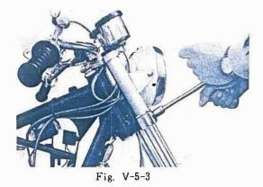
4) Pull the outer tube downward
