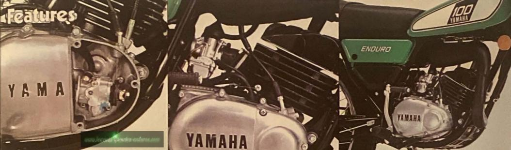
Autolube monitors engine load and speed then auto-matically mixes oil and fuel accordingly. Constant flow adjustment to meet operating conditions helps extend engine life.
