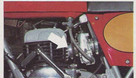
This manufacturer has a Torque Induction® type reed valve on his factory motocrosser. But not on his production bikes.
