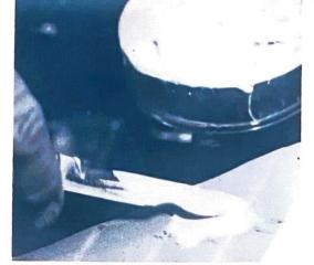
Hole readied for patching with the hand grinder. Next step is to apply epoxy or fiberglass patching compound. The latter is simply fiberglass resin with finely chopped fiberglass already added. Because the Alpina has a painted tank, I smoothed the patch carefully while the repair compound was still soft, thereby eliminating sanding.
