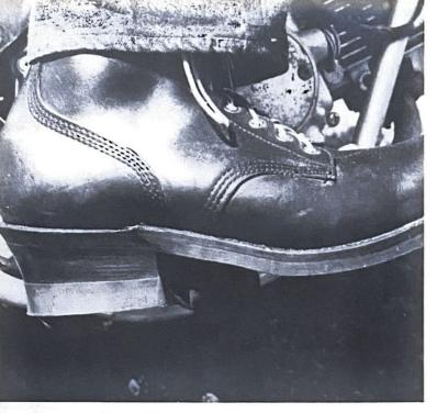
An extremely poor boot design for trail riding. High, square-front heel is a cinch to catch on something — one of the easier ways to break a leg! A little manicuring with a hacksaw would work wonders here.
