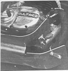
Bultaco Pursang equipped for desert racing with a Bill Water's rock guard to protect the down pipe from minor bumps. For enduros or true rocky going it is a better idea to switch to a high pipe and gain ground clearance — without the rock guard.
