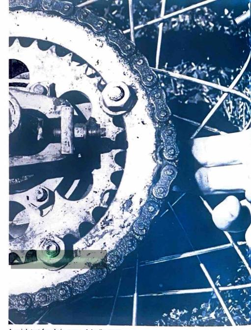
A quick test for chain wear. A badly worn chain will pull away from the back of the sprocket almost to the height of the teeth. This chain is in quite good condition and has about 1000 off-road miles on it.
