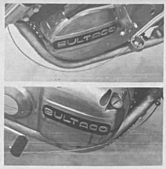
Brush guards on Bultaco's Matador "Six-Days" model are cables attached from the frame cradle to the shift and brake levers. Note that the cable fastens to the outer edge of the shift lever and that brake lever is rounded to make it less likely to hang up on rocks or in brush. Shop rag contains tools. Dave Ekins photo.
