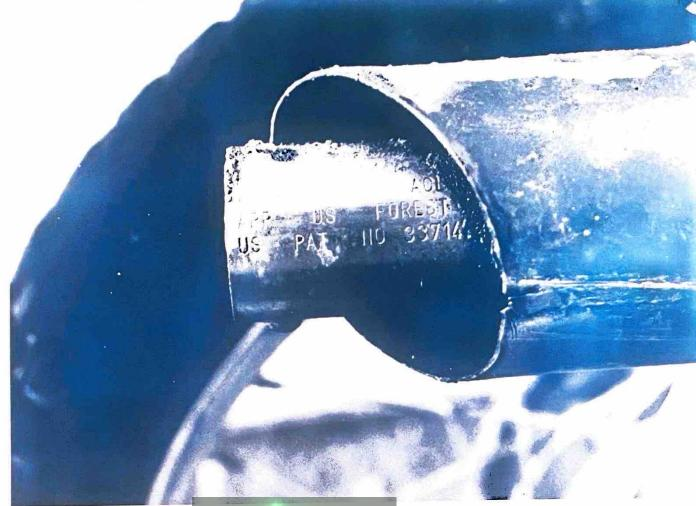
If you're going to be riding on public land or anywhere that spark arrestors are required, make sure your new bike comes ready-fitted with a USDA-approved arrestor in addition to the muffler. This one is on a Hodaka B.
