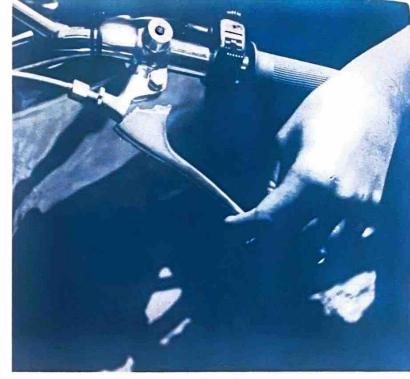
There are places you don't use Loctite and this is one of them. Danny persisted in tightening his lever clamps excessively — and broke two levers in two days as a direct result. He started adjusting them so that they were just tight enough to keep from working around the bars of their own accord. And hasn't broken one since!
