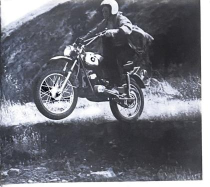
Although not very high, this bank is still too high to simply ride over because the frame would hit when the front wheel dropped over. Slack in lower run of chain indicates power is still being applied to keep the front wheel slightly above the horizontal. Danny is keeping his weight well to the rear to keep the front wheel up.
