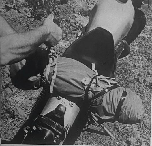
When packing the ground-cloth-wrapped Ensolite pad on the bike I have found it pays to add electrician's tape keepers to the nylon tape to keep the lashings from working. As Ensolite has a "memory" it should not be lashed too tightly or permanent scars will be left — hence the black tape.
