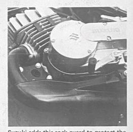
Suzuki adds this rock guard to protect the down pipe on their 175 cc model. Still, it affords only minimal protection. So, if you get really serious about riding in the rockery — install an up pipe.
