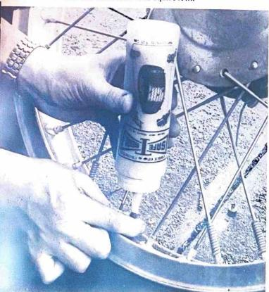
experienced pavement riders use the valve cap because at high speed centrifugal force coupled with the normal jouncing from the pavement will lift the valve from its seat, allowing the tire to deflate. This is not too severe a problem until the bike slows.
