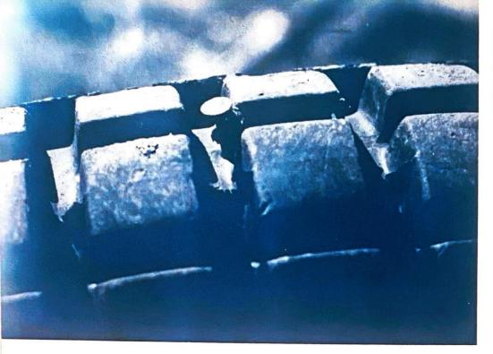
But sometimes the cause of the trouble is painfully apparent. I discovered this nail as I was rolling the bike into the garage, although the tire never actually went flat, thanks to Safe-T-Seal. This tire has about 800 off-road miles on it.
