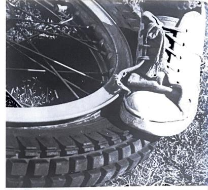
Before setting-to with the tire irons 'break' the bead loose from the rim by tramping it down
