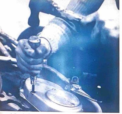
A 'knocker' or Impak Driver is an absolute necessity for working on bikes with Phillips-type screws. These work best with a hammer of 16 to 20 oz, and all our ball-pein hammers are either too heavy or too light, so we borrowed the carpenter's beater from the kitchen mechanic.
