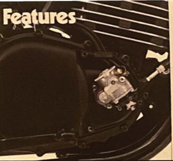
Autolube," a feature on most Yamaha two-stroke engines, automatically injects oil into the fuel mixture, eliminating the need for premixing. And, since it adjusts the flow of oil to engine load and speed, it extends engine life.
