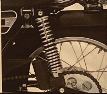
Thermal-Phase rear shocks have built-in oil coolers to prevent overheating, no matter how hard or long you ride.
