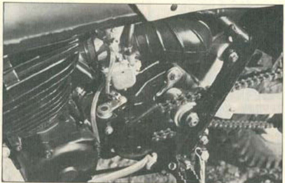
Protective chain rollers abound. Bits of plastic and nylon nudge and guide the chain from end to end.
