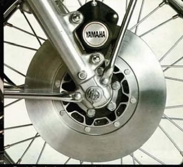
Front disc brake stops you faster. An adjustment screw lets you set the hand-lever for the exact "feel" you prefer. The enduro-type front forks will soak up the hardest jolts and resist bottoming.
