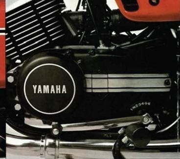
Six-speed transmission keeps the engine running at its most efficient speed. The short-throw shift lever lets you change gears quickly, without lifting your foot from the peg. Yamaha gearboxes are notoriously runged.
