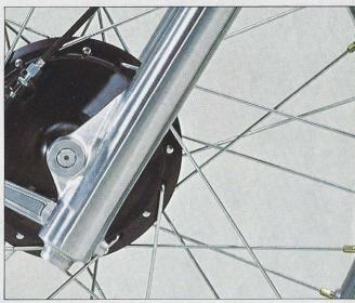
The leading axle design allows quicker, more precise low-speed steering. In addition, the damping characteristics can be improved through the increased oil capacity of the fork tube.
