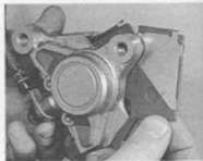
Remove pads from caliper noting correct positions of anti-squeal shims
