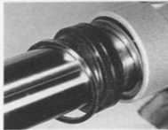
3.19 DT model - oil seal, washers, dust seal and top bush should be removed with stanchion
