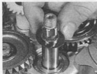
41.1a Fit dished washer to input shaft right-hand end ...
