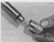
3.5b Place damper rod seat over damper rod end ...
