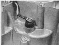
14.5a Neutral switch lead must be disconnected ...
