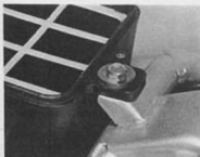
4.2b ... then remove mounting bolt and remove complete air filter assembly from machine
