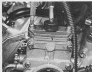
4.10 On flat-slide carburettor the top is retained by two screws
