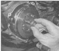
5.1a A large washer is fitted behind the generator rotor centre nut
