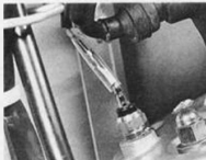
4.11b Disconnect temperature sender lead and suppressor cap
