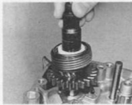
40.3a Install kickstart assembly ensuring friction clip is correctly located in recess provided in casing ...
