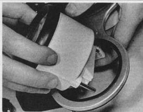
17.2d Instrument heads can then be removed from panel
