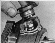
43.2b Refit sleeve and end cap assembly ...
