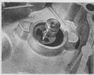
14.9b ... and secure it with a circlip as shown
