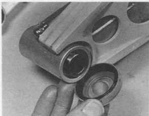
11.9b ... which fit inside thrust caps
