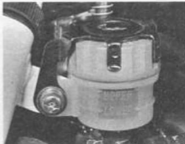
...and rear master cylinder reservoir ensure level does not fall past lower mark
