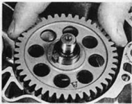
38.2c Fit balancer shaft drive gear making sure punch mark faces outwards ...
