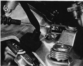
45.7a Connect clutch cable to lifting arm and bend up tab (arrowed)
