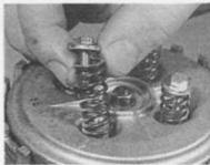
41.5b Refit springs and retaining bolts and tighten them to the specified torque setting
