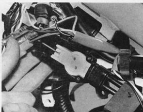
DT model - examine throttle cable junction box if pulley does not operate smoothly
