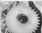
9.6c ... and refit second plain washer, securing them both with a circlip
