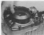
42.2 Rotate crankshaft whilst refitting cover to ensure oil and water pump drive pinions engage correctly
