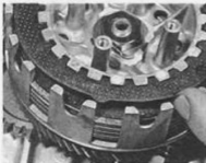
41.4 Note cutaway area on plain plates. These must be arranged as described in text
