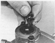
7.3a Slacken and remove left-hand valve cap centre bolt followed by the valve cap itself
