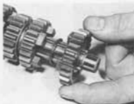
30.6e Slide on the 6th gear pinion ...
