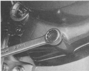
Transmission oil drain plug is situated at bottom of right-hand crankcase cover
