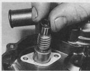
14.6 Do not omit shim when refitting oil pump and use a new gasket
