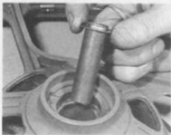
6.8a Fit first wheel bearing then invert wheel and fit central spacer - grease cavity ...
