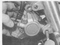
To remove brake pads, remove caliper mounting bolts (TZR 2RK and 3PC1 models) ...
