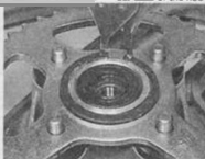
7.2b ... followed by large circlip ...
