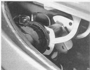
2.8 On refitting ensure tank engages correctly with rubber buffers — TZR model shown
