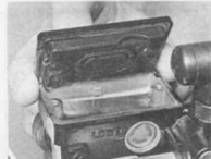
Ensure that diaphragm is correctly positioned before refitting brake fluid reservoir cover
