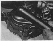
9.6e Refit cover and tighten retaining screws to specified torque setting
