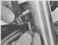
2.2 Release brake hose clamp from fork leg - TZR model shown
