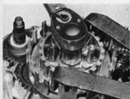
41.3a ... and tighten nut to specified torque setting whilst holding clutch centre as shown
