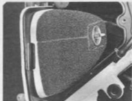
... withdraw filter assembly
