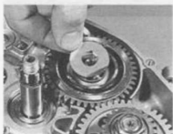
38.4a Fit a new tab washer ...
