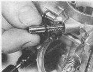
5.9b ... and pilot screw for signs of wear or damage
