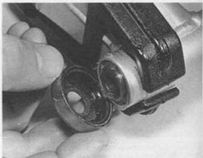
12.1b Grease inside of thrust caps before refitting them to the swinging arm
