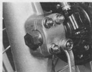
3.4b DT model – check spindle clamp is correctly fitted (arrow facing up) and tighten nuts as described in text
