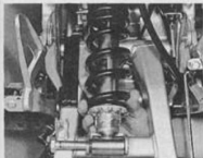
13.3a TZR model - withdraw suspension unit lower mounting bolt ...
