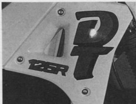
2.1 DT model - air scoops are retained by three screws
