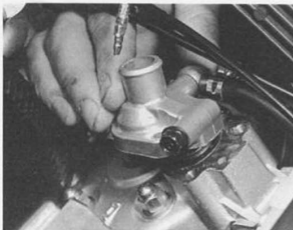
8.4a Remove thermostat housing screws and lift housing clear
