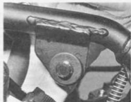
4.7f ... and rear mounting bolts and manoeuvre exhaust clear of frame
