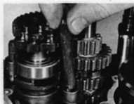
33.4c Refit selector forks into their respective slots in the drum and install selector fork shafts
