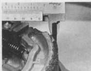
14.2a Brake shoe lining thickness measurement
