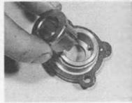
43.2a Ensure slot on brass sleeve locates with peg on inside of left-hand end cap
