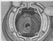
14.3 Fold brake shoes together in a 'V' to permit removal
