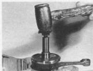
33.1 Fit crankshaft and gearbox components into left-hand crankcase half - do not use excessive force when refitting crankshaft
