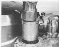
9.4c If necessary drift seal into position using a suitably sized socket
