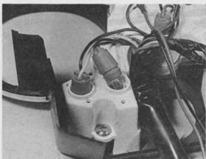
14.4 Instrument and warning lamp bulbholders are a press fit in panel assembly
