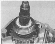
40.3b ... then engage the kickstart return spring into its locating hole
