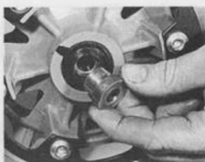
3.1b ... and spacer – TZR model shown
