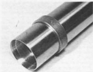
3.22 Oil top bush liberally before sliding into place
