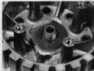
41.2d Fit a new tab washer ...
