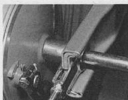
5.1c On drum brake models install right-hand spacer whilst inserting wheel spindle
