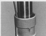
3.4b Prise out oil seal retaining circlip using a small screwdriver
