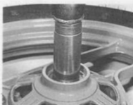
6.8c ... using a hammer and tubular drift
