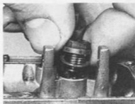
5.2e Remove the needle seat as described in text - early type carburettor shown
