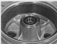
14.2b Drum surface must be free from brake dust and scoring
