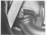
4.7d Release two front mounting nuts ...
