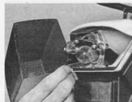
14.6d The DT model lamp lens is retained by two screws and uses a single bulb ...
