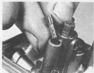
5.4a Pilot jet can be removed using a slim narrow-bladed screwdriver
