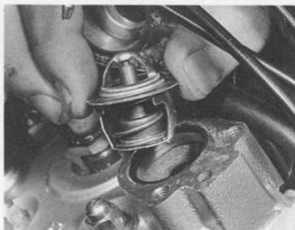
8.4b Thermostat can then be removed along with O-ring
