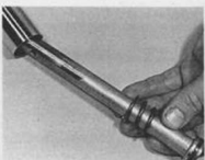
3.9a Fit rebound spring to damper rod and insert into stanchion upper end
