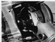
44.2b Ensure dowels are in position (arrowed) and fit a new gasket
