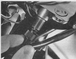
17.2b Release drive cables ...
