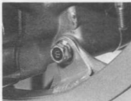
4.15a TZR125 – to release engine, remove front mounting bolt and spacer
