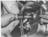
5.9a Remove and examine throttle stop ...
