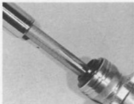
3.9c ... and insert stanchion assembly into lower leg
