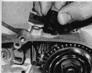
39.1a Fit driven gear and plastic housing. Avoid overtightening the retaining bolt
