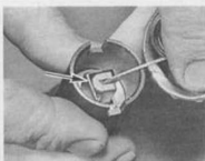
4.5 To remove throttle valve, compress return spring and shake out spring seat (arrowed)
