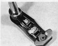
37.2 Ensure gear change shaft return spring is correctly fitted
