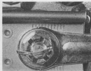
5.2a Tighten spindle nut to specified torque setting and secure with a new split pin
