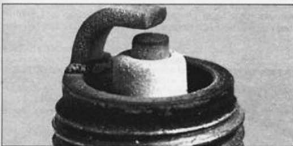
Normal condition - A brown, tan or gray firing end indicates that the engine is in good condition and that the plug type is correct
