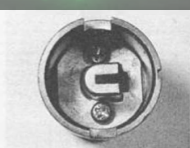
5.5 Needle is retained by a plate inside throttle valve
