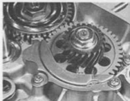
38.5 Fit oil baffle plate having first applied thread-locking compound to its retaining screws
