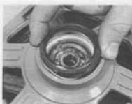
6.9c Grease seal to aid installation
