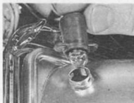
14.2d Parking lamp bulbholder is a bayonet fit in headlamp unit
