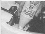
Use only good quality two-stroke oil when topping up - TZR model shown
