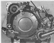
42.3 Do not omit oil pipe clamp or breather hose guide when refitting retaining screws
