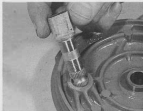
14.5a Apply a smear of high melting-point grease to brake camshaft prior to refitting ...
