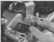
13.3b ... followed by upper mounting bolt and remove unit
