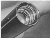
3.13 Ensure circlip is correctly located in its groove
