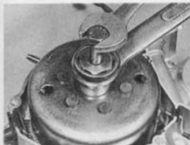
14.4 Extractor must be used to remove rotor
