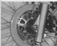
On DT models remove disc and caliper covers to gain access to front caliper
