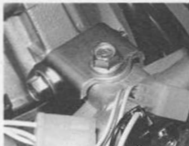
4.16 Remove both rear mounting bolts and top engine mounting/frame bolt
