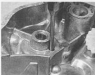
9.4a Drift out water pump seal via hole provided in crankcase cover
