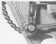
On drum brake models, adjust rear brake at end of operating rod
