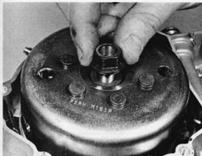
36.3a Fit rotor followed by plain washer and nut ...
