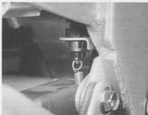
8.7 Rear stop lamp switch location - TZR125 shown
