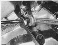
4.9 Slacken clutch cable adjuster and disconnect cable
