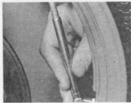
Ensure tyres are run at the correct pressure...
