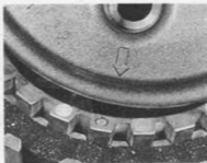
41.5a Align arrow mark on pressure plate with circular mark on clutch centre and fit pressure plate
