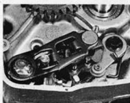
37.4 Check the operation of the external gear selector components as described in text
