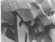
On TZR model brake caliper must be viewed from rear to check pad wear
