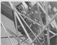
3.2b DT model – position disc correctly between brake pads whilst refitting wheel
