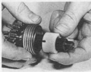
40.2d Slide nylon guide into place ensuring that notch engages with inner end of kickstart spring
