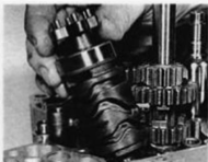
33.4b Swing forks away to provide clearance for selector drum to be installed
