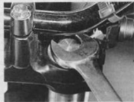
2.4c DT model - slacken top bolt while fork leg is clamped in the yokes, if fork legs are to be dismantled
