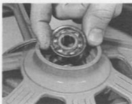
6.8b ... and fit second bearing ...
