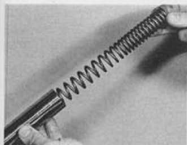
3.4a TZR model - note which way up fork springs are fitted on removal
