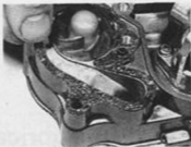
9.6d Check locating dowels are in position and fit a new gasket
