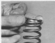
3.25a Refit fork spring and spring seat ...
