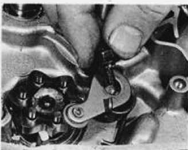
37.1 Apply thread-locking compound to shouldered bolt and refit detent arm and return spring
