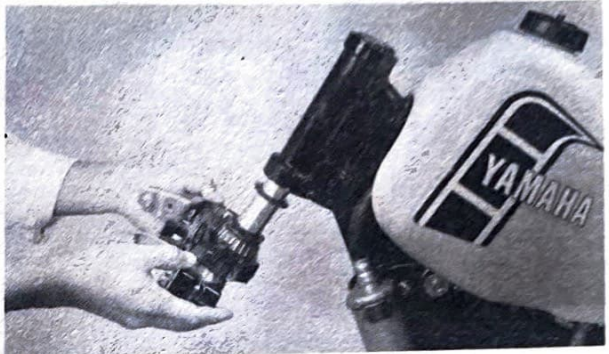
12. Remove the under bracket, lower bearing and oil seal.
