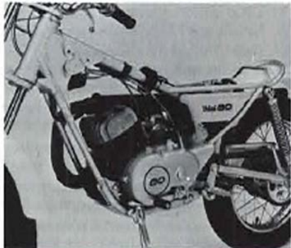
The double-cradle tubular frame has been designed more slim, but, with higher flexible strength, making it ideal for swiss and turns in a tough trials section.
