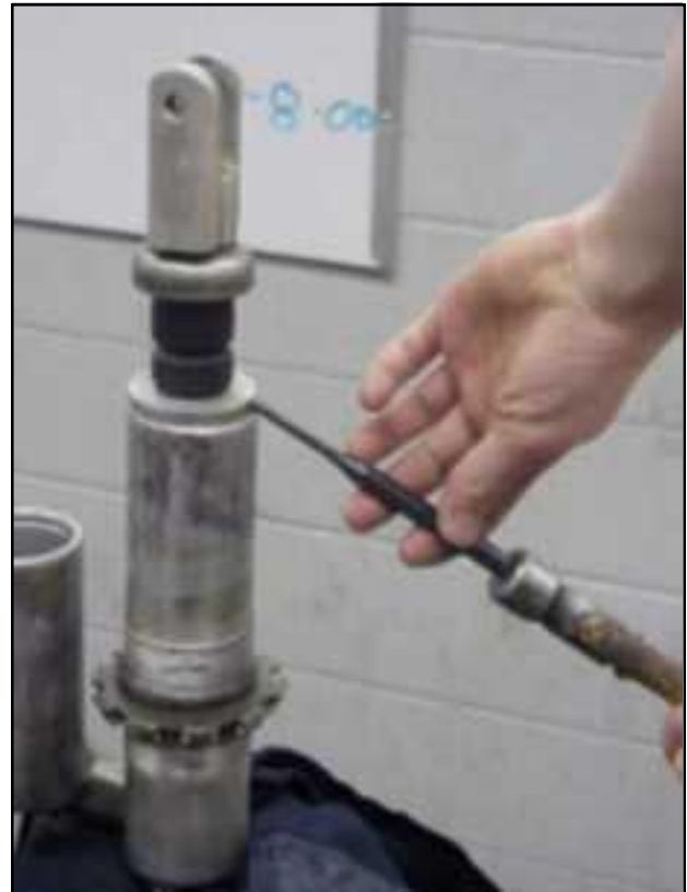
Fig 4 Tap the shock body end cap up.
