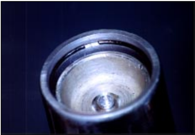
Fig 2 Push down the bladder cap until the circlip is exposed.
