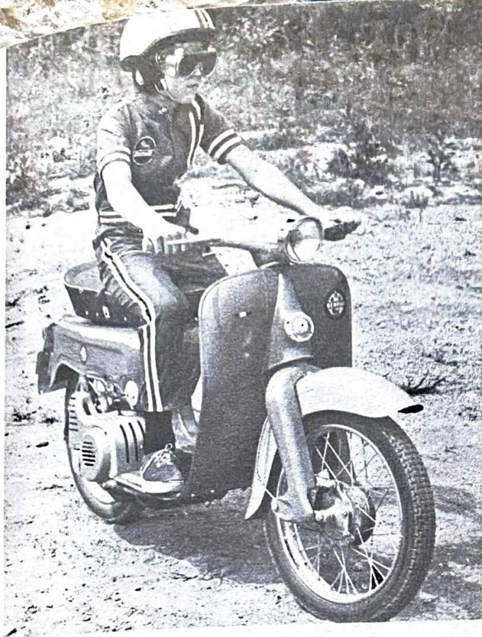
A rider is maneuvering a Benelli scooter at slow speed, has pulled the clutch, and is ready to shift to next gear.
