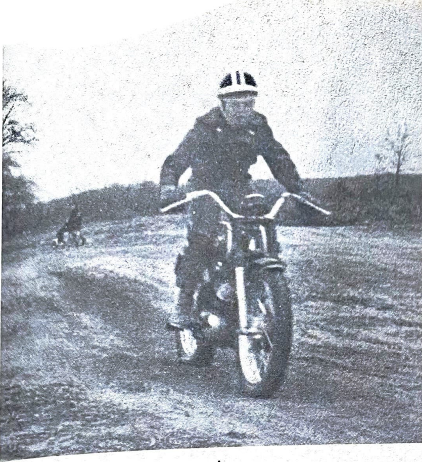
Bike should be landed on the rear wheel, and rider should be off the seat. Note deflection of rear tire.
