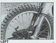
Up front are a good set of forks. Not as responsive to little bumps as we'd like, the way our test bike was set up (see test), but good. The front guard is excellent, the headlight detach system is the best in the world, and Yamaha's twin leading shoe front brake is great once you use it a couple of times.
