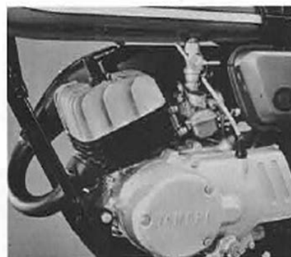
Valve induction system increases the "effective" horsepower delivered to the rear wheel.
