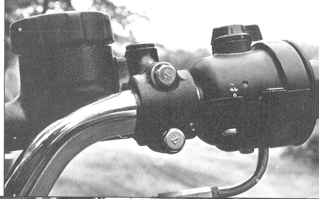
Switches on the right side of the bar accommodate the headlamp and an ignition "kill."
