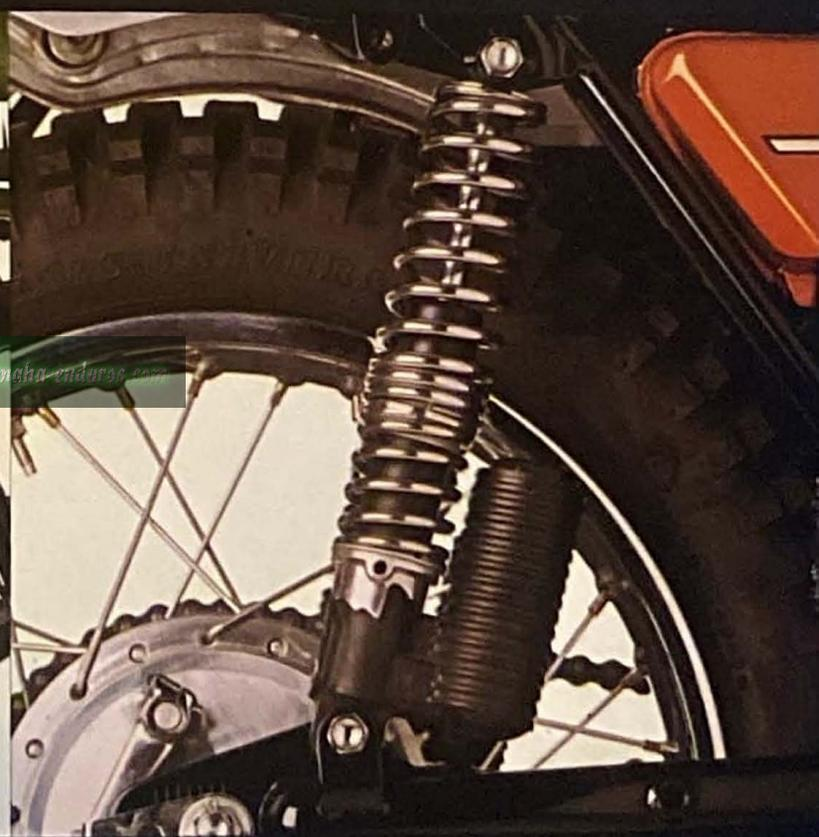
**Thermal-Phase rear shocks** have built-in oil coolers to prevent overheating, no matter how hard or long you ride. Interchangeable jets also allow you to adjust compression and rebound characteristics individually.
