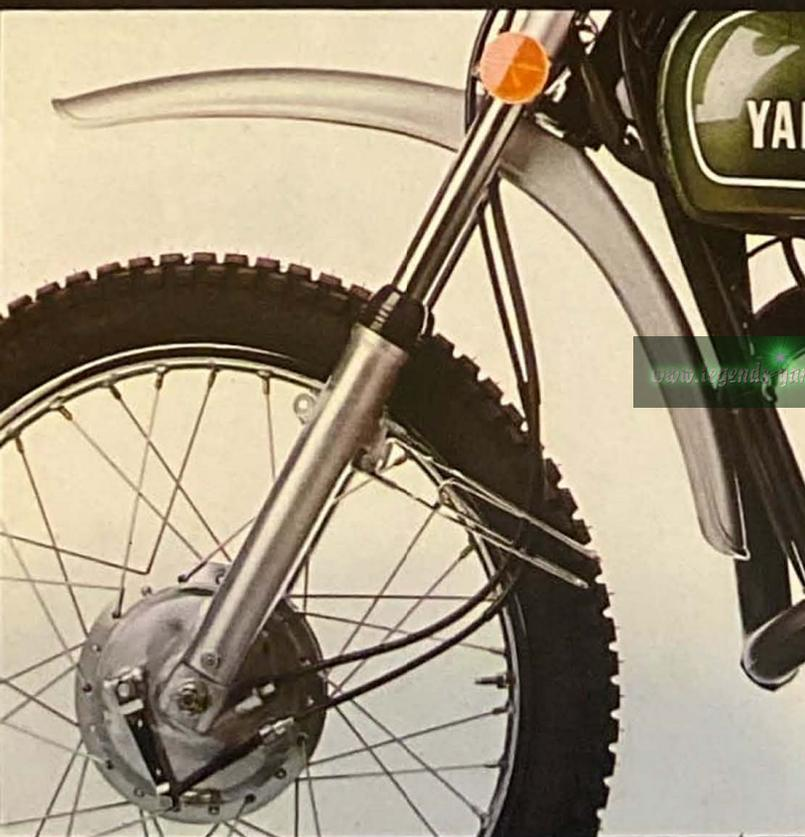
**New high-clearance fender** of lightweight polypropylene is virtually unbreakable. New front fork design and new steering geometry help 1974 Yamaha Enduros handle like motocrossers on rough trails.
