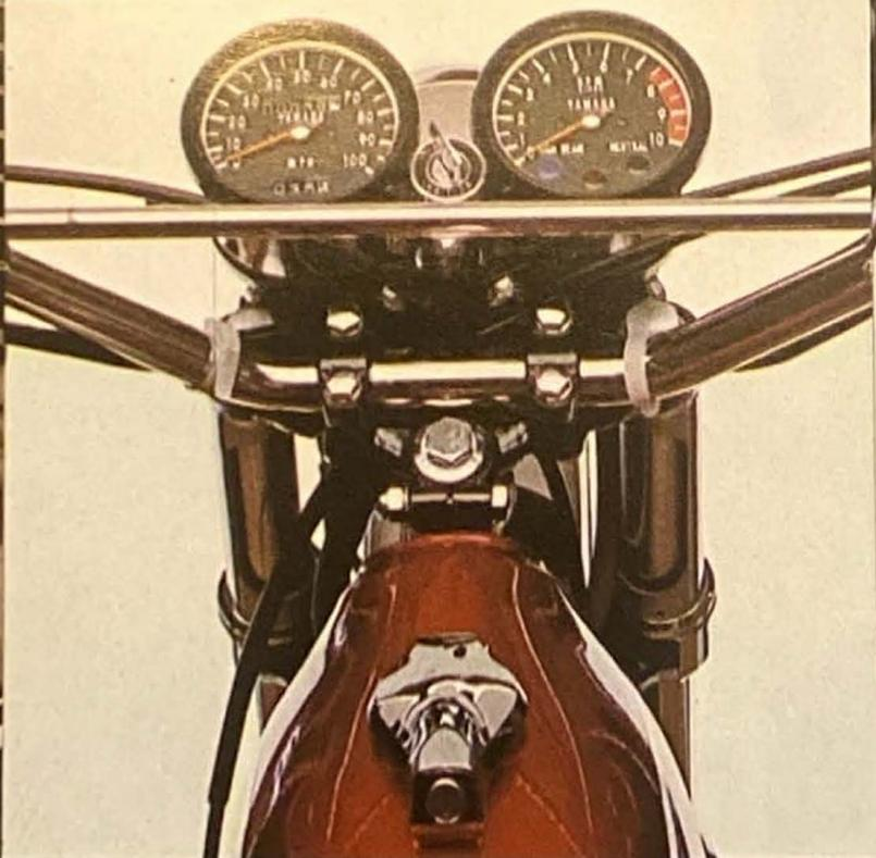
**Enduro-type instruments** include speedometer, tach, and resettable trip odometer. A single key locks ignition, forks, gas cap, and accessories compartment. Complete lighting system makes Yamaha Enduros fully street legal.
