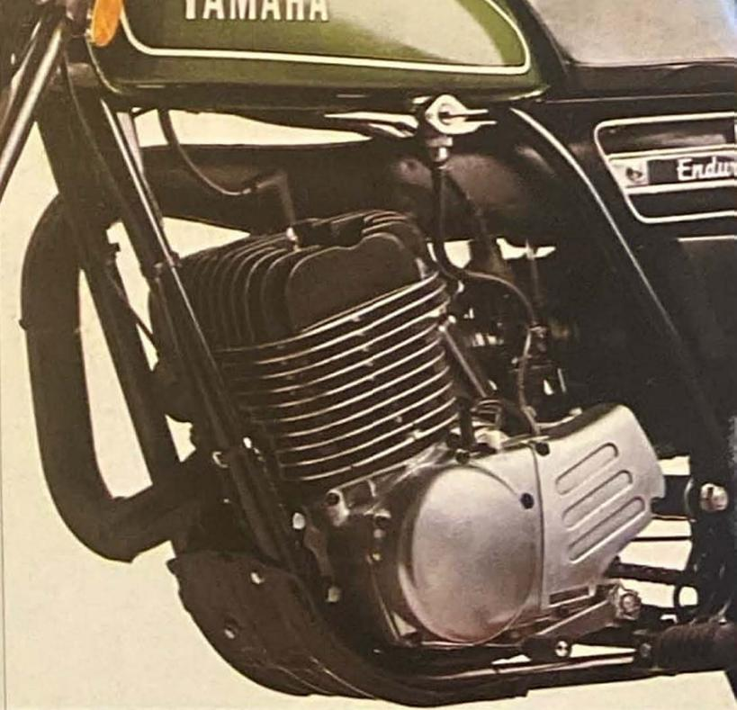
**Motocross-type frame** cradles the engine lower, has lower center of gravity for better handling. This new frame design, adapted from the highly successful Yamaha motocrossers, also flexes less, for surer tracking.
