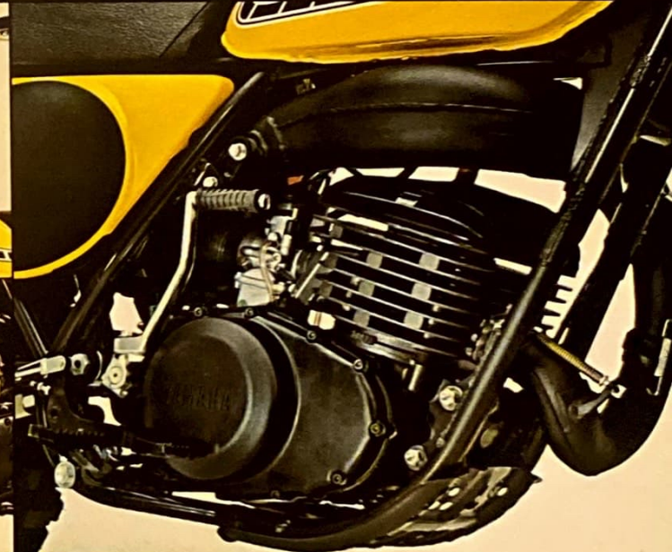
Double loop frame has a low profile. That low center of gravity provides better balance for easier handling.
