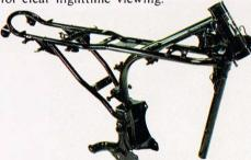
Utilizing the experience gained from the world's most demanding motocross tracks, YAMAHA has developed a lightweight, tubular-steel, single-down-tube frame that is able to give the machine an overall lower center of gravity for better maneuverability. This high-tensile-strength steel frame is designed to withstand the stresses and strains which are absorbed from the roughest of roads in order to assure long-term durability and stability.
