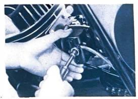
After replacing the main jet, check the engine operating condition in the following manner. Rapidly open the throttle valve, and observe the increase of the engine speed. If the speed will not increase smoothly, showing irregularity, the position of the jet needle must be changed.
