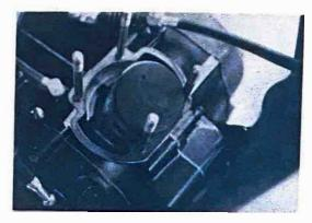
d. Tighten the cylinder head nuts cross-pattern and in separate steps. Tighten torque must be correct.
