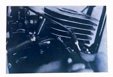
e. Loosen the air cleaner joint band.
