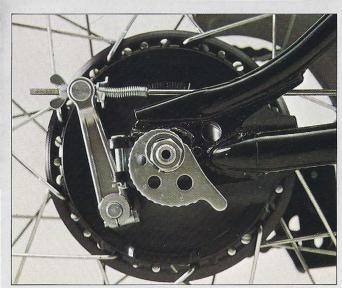
Chain-adjusting cams allow rapid rear wheel alignment when adjusting the drive chain or after removing the rear wheel.
