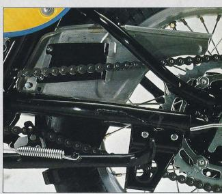
Chain shield keeps mud and sand from being thrown into the chain. Increases chain life.
