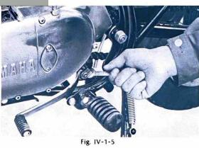
4. Remove the chain cover, and then disconect the clutch cable.
