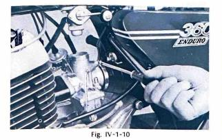
9. Disconnect the oil line at the bottom of the oil tank.
