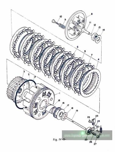
1. PRIMARY DRIVEN GEAR COMP. 2. O-RING 3. BOSS, Clutch 4. PLATE, Clutch (1) 5. RING, Cushion 6. PLATE, friction 7. PLATE, clutch (2) 8. PLATE, pressure 9. SPRING, clutch 10. SCREW, spring 11. ROD, push 12. BALL 13. NUT, lock 14. SPRING, bellevile 15. SPACER 16. BEARING 17. PLATE, thrust (2) 18. PLATE, thrust (1) 19. ROD, push 20. PUSH LEVER ASS'Y 21. SPRING, return 22. HOOK, spring 23. JOINT 24. PIN 25. PIN, cotter 26. SCREW, adjusting 27. NUT, adjusting
