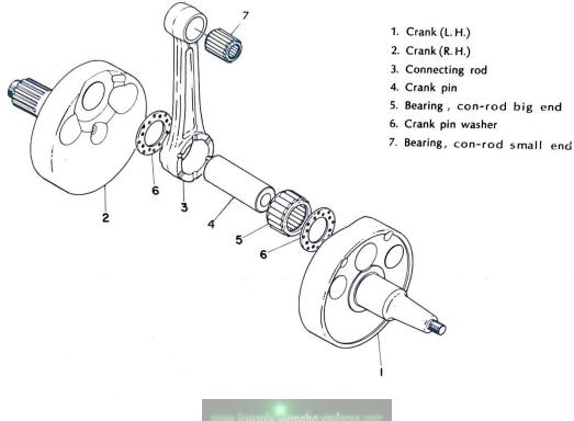
Fig. IV-16-2 Crankshaft component parts
