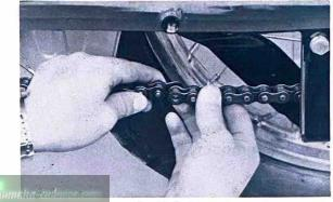
Loosen the chain tension adjusting nuts and bolts on both right and left sides.
