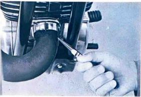
2) Remove the muffler holding bolts. (Figs. IV-1-3 and 4)
