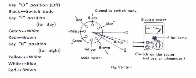
If the readings or the above six meaurements are nearly  $0 \Omega$ , and no shortcircuit is noticed between the terminals, as well as between the lead terminal and the switch body, the main switch is in good condition.
