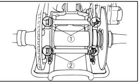
1. Upper wheel hub bolt (×2) 2. Lower wheel hub bolt (×2)
