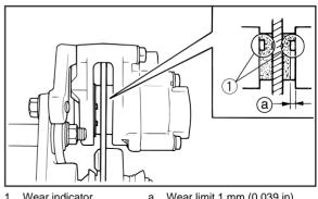
Wear indicator Wear limit 1 mm (0.039 in) a.
