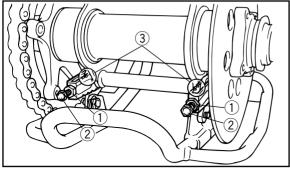
1. Locknut 2. Chain adjuster 3. Alignment marks
