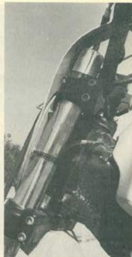
The nitrogen, or nitrogen valve, sticks out of the frame through a hole that you must drill. Be sure to follow the instructions. It is murder to get that little braided hose through the hole.
