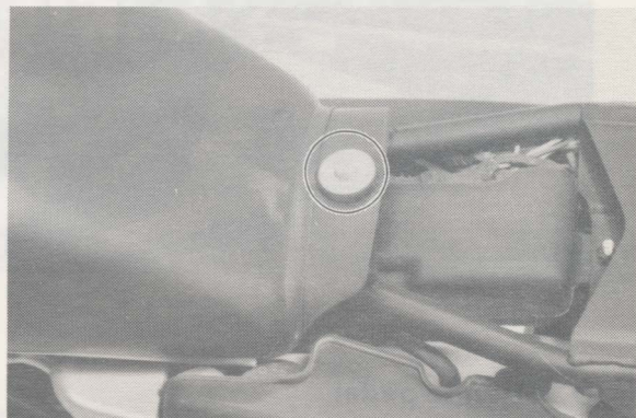
1. Fuel tank holding bolt
