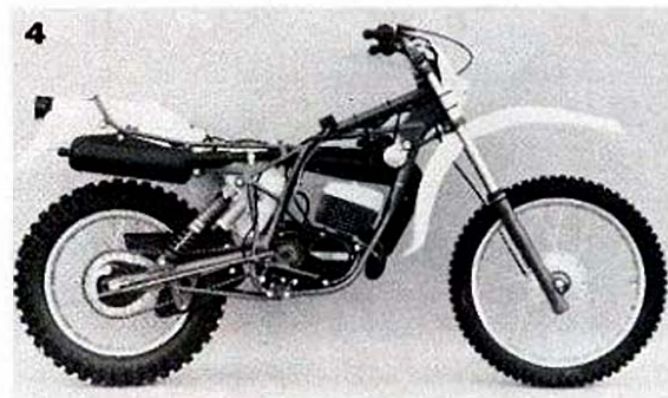
The Hercules' well-triangulated, massively-gusseted chromoly frame (1) is probably the strongest of the five. The mild-steel Can-Am frame (2) also is quite strong due to its large main backbone and surplus of triangulating tubes, but both it and the Herc frame could be made lighter. The mild-steel PE175 (3) and chromoly SWM (4) frames are light and simple, yet sufficiently strong. The mild-steel Yamaha frame (5) is light but has no direct swingarm-pivot-to-steering-head bracing. A massive, stamped steel backbone gives the structure adequate rigidity.
