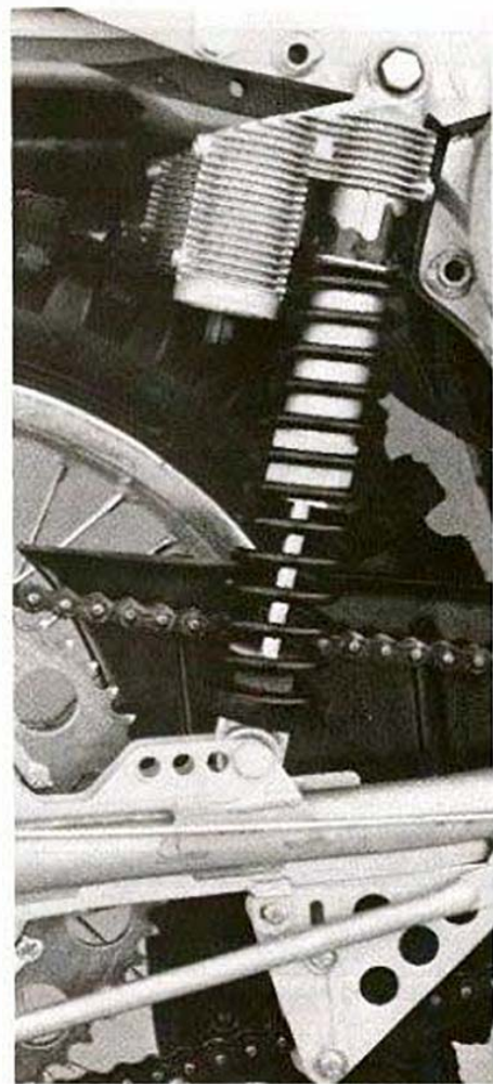
The Hercules offers a multitude of rear shock mounting positions. As far as we're concerned, the best springing/damping/steering-geometry/ground-clearance combination is obtained with the Marzocchis attached as you see them here.
