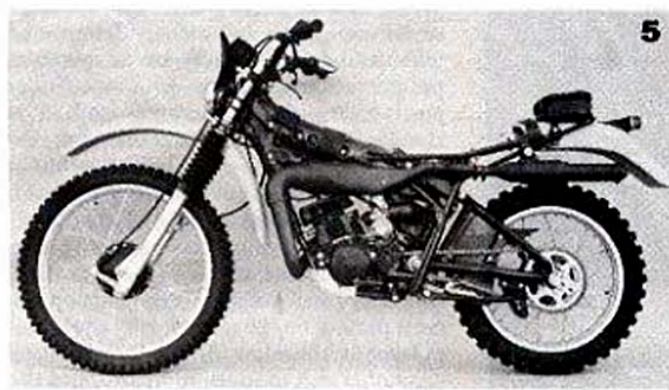
The Hercules' well-triangulated, massively-gusseted chromoly frame (1) is probably the strongest of the five. The mild-steel Can-Am frame (2) also is quite strong due to its large main backbone and surplus of triangulating tubes, but both it and the Herc frame could be made lighter. The mild-steel PE175 (3) and chromoly SWM (4) frames are light and simple, yet sufficiently strong. The mild-steel Yamaha frame (5) is light but has no direct swingarm-pivot-to-steering-head bracing. A massive, stamped steel backbone gives the structure adequate rigidity.
