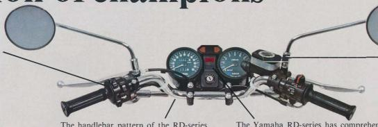
The master cylinder for the hydraulic disc brakes is mounted on the right handlebar. It has translucent sides so that the vitally important fluid level can be visually checked with one quick glance.
