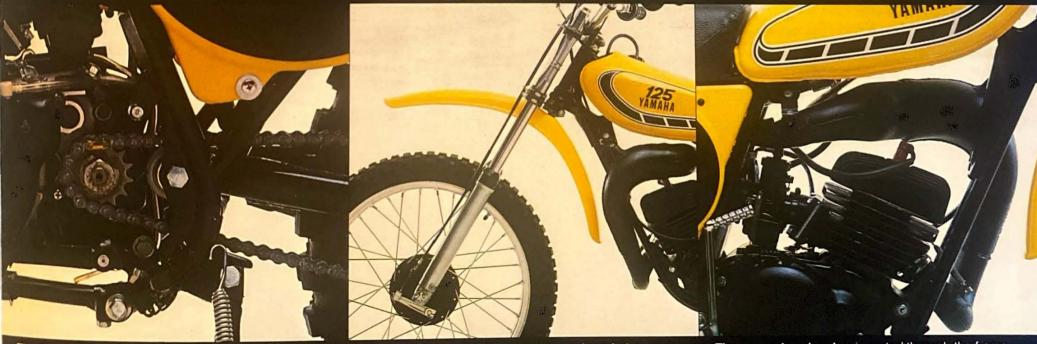
The 6-speed transmission allows you to get the most possible horsepower to the ground under all conditions. Like all Yamaha transmissions, it features a drum type shift cam that provides positive shifting. The new YZ125 uses the same strong front forks as our larger YZ models. They provide over 7 inches of travel. The expansion chamber is routed through the frame where it is out of the way. The result is an extremely narrow profile, low engine position and good ground clearance.
