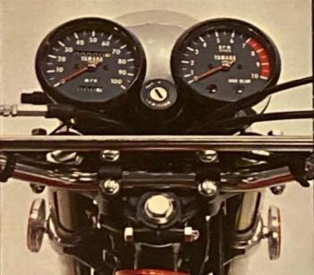
Enduro-type instruments include speedometer, tach, and resettable trip odometer. A single key locks ignition, forks, gas cap, and accessories compartment. Complete lighting system makes Yamaha Enduros fully street legal.
