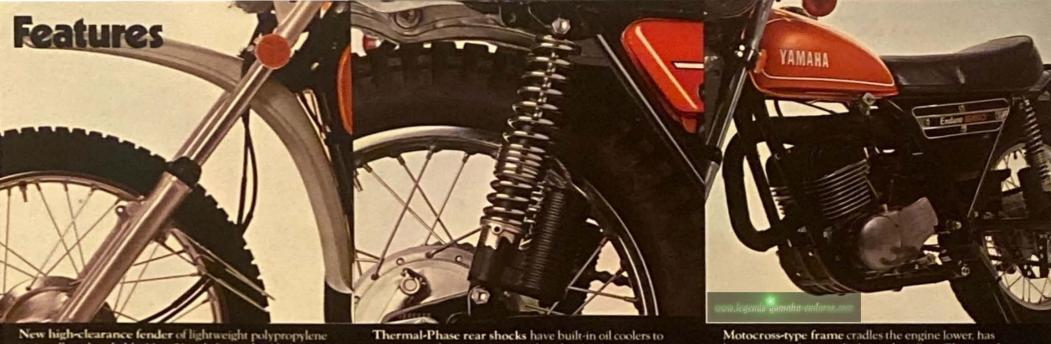
New high-clearance fender of lightweight polypropylene is virtually unbreakable. New 21 inch front wheel helps maintain steering control on rough terrain.
