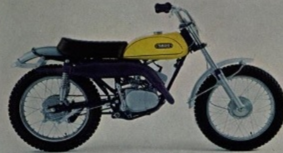
125 AT-1MX With a close-ratio 5-speed gearbox, Gyt Kit, tuned exhaust and Autolube, you can look for this one in the winner's circle.
