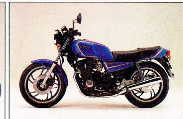
XJ650 Featuring a narrow in-line four cylinder DOHC 4-stroke motor, the XJ650 is one of the slimmest mid-range machines available.
