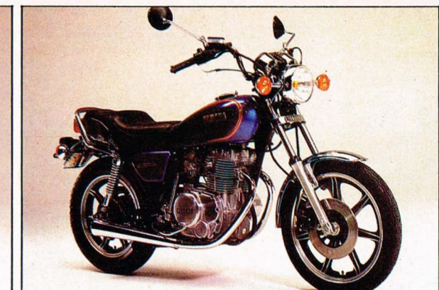
XS250SE Featuring an economical and reliable 4-stroke twin cylinder power unit with electric starting, the XS250SE has US custom styling giving a casual, comfortable riding position.
