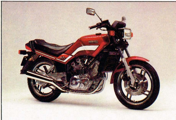
XZ550 A 70° V-twin liquid cooled DOHC 8 valve power plant, monocross suspension and shaft drive makes the XZ550 a super smooth middleweight winner.
