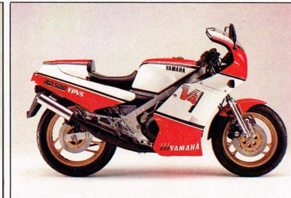
RD500LC Direct descendant of Kenny Roberts' YZR500 factory racer, featuring Yamaha's power valve system, new monocross suspension, aerodynamic full fairing and anti-dive front suspension.
