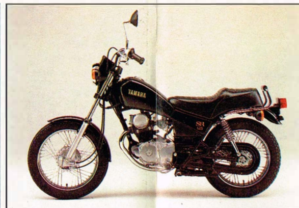
SR125SE Featuring an economical 125cc SOHC 4-stroke motor with comfortable riding position, the SR125SE offers semi-enclosed rear chain and electric starter.
