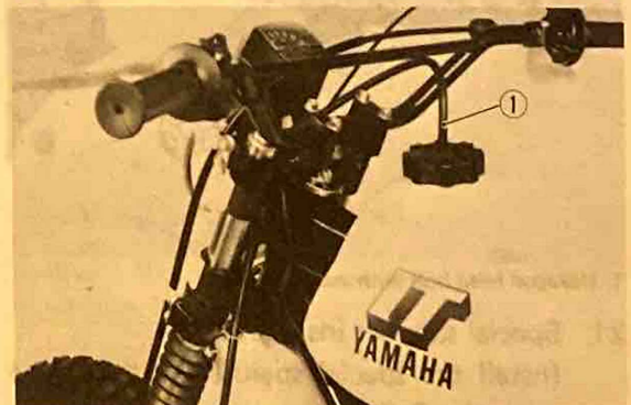
1. Fuel tank breather pipe (D-7)
