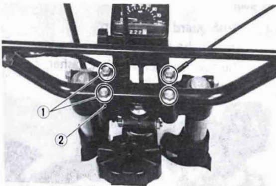
1. Flange bolt (C-2) 2. Upper holder (C-1)
