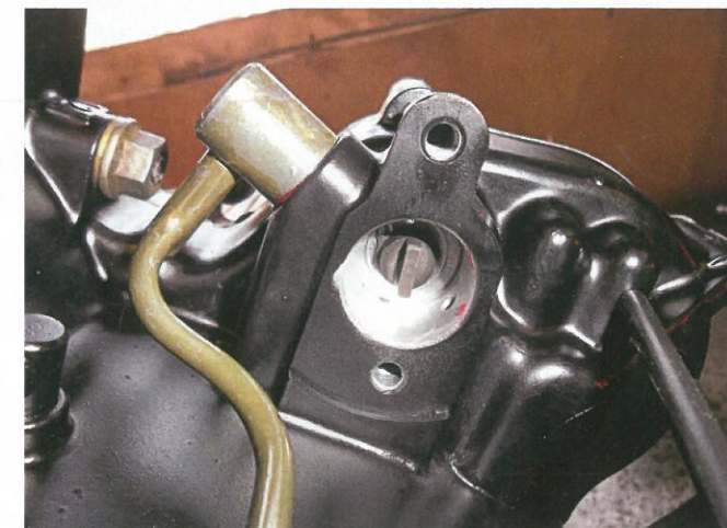
Now line up the drive peg with the bolt holes.
