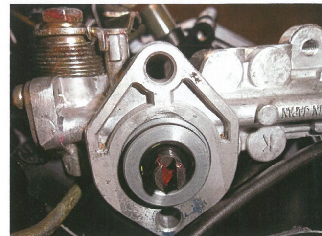
Here I line up the drive slot with the bolt holes.
