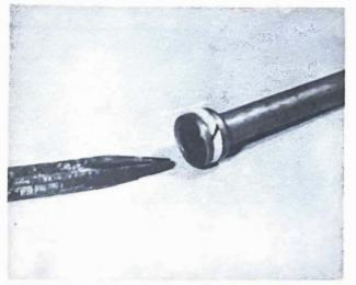
4.3a Tapered dowel or rod will prevent damper rotation ...
