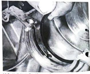
28.2a Half ring is fitted into crankcase groove ...
