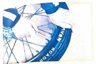
Tyre removal: Deflate inner tube and insert lever in close proximity to tyre valve
