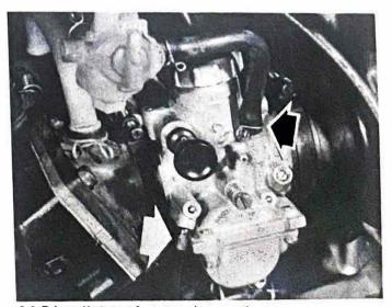
6.2 Prise off oil and fuel pipes (arrowed)
