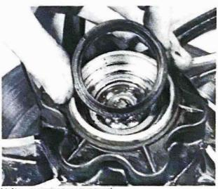
11.1b ... and prise out grease seal
