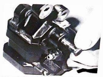
4.6b ... and withdraw pin to free caliper bracket
