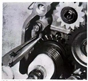
10.2a Unhook the kickstart return spring from its anchor pin
