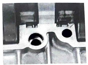
26.3a Centre bearings are located by small pins ...
