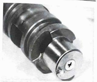
20.8e Neutral switch contact is secured by plate and screw
