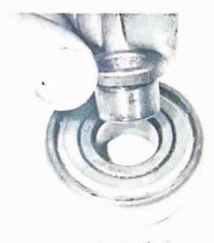
12.1f Fit short spacer into bearing as shown ...
