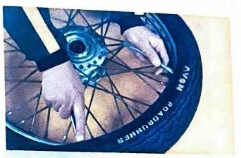
Use two levers to work bead over the edge of rim
