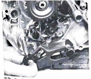
30.2b ... then slide selector mechanism into place
