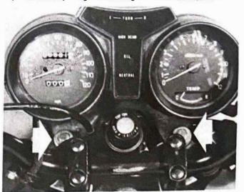
3.3 Instrument panel is retained by two bolts
