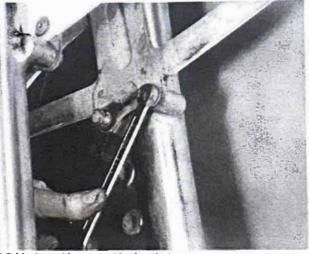
2.3 Mudguard is secured by four bolts
