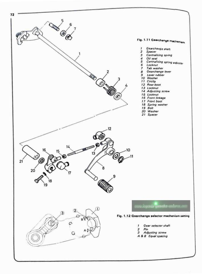
30 Engine reassembly: fitting and adjusting the gear selector shaft
