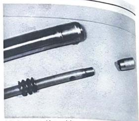
5.1 a Check stanchion and damper parts for wear
