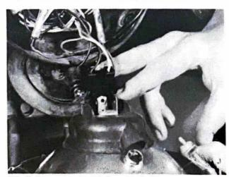
9.2a Bulb connector is push fit on terminals
