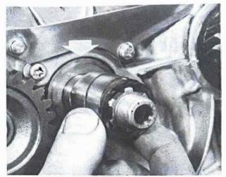
32.3a Fit large thrust washer (arrowed) and clutch bush
