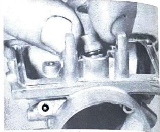
7.5b ... and withdraw float valve seat
