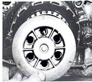
32.6d Clutch pressure plate can now be fitted ...
