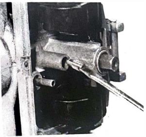
7.4b Pilot jet is fitted into adjacent drilling
