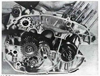
11.3 Release crankcase bolts and separate crankcase halves
