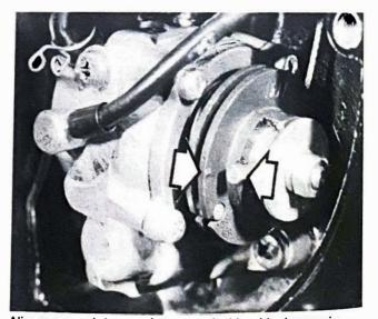
Alignment mark (see text) should coincide with plunger pin
