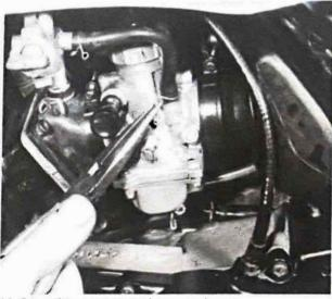
4.5a Prise off the petrol feed pipes at carburettors
