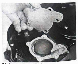
7.3a Pump cover is secured by five screws
