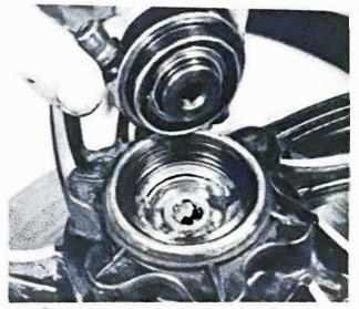
11.1a Remove speedometer drive gearbox ...
