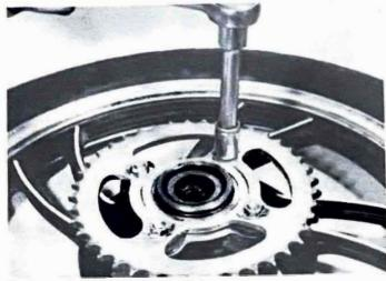
14.2c ... the four sprocket retaining nuts
