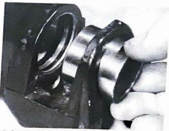
4.5b Displace piston and remove from caliper body
