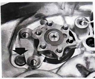
26.5a Note that retainer plate locates shaft (arrowed)
