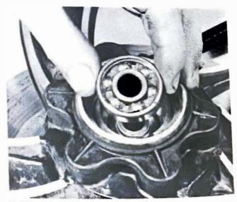
11.5d ... grease and install remaining bearing
