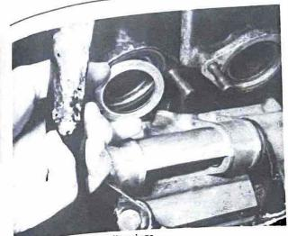
35.8a Fit exhaust port sealing rings ...
