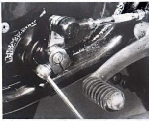
35.5d ... and secure front of linkage to shaft
