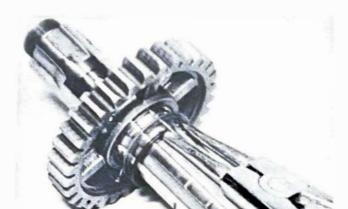
14.7a Output shaft has plain shoulder at sprocket end
