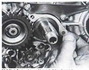
31.3 Fit deflector plate and input shaft bearing retainer
