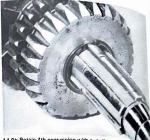
14.9b Retain 4th gear pinion with a circlip
