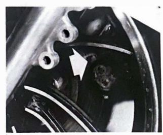
9.6a Check that disc engages pads as shown ...
