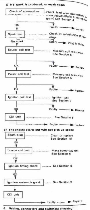
1 The single most likely cause of ignition failure or parial failure is a broken, shorted or corroded connector, switch contact or wire. Tracing faults of this nature can often prove time consuming but does not require the use of sophisticated test equipment. Although in rare instances a particular fault will not be evident from a physical examination, it is worthwhile
