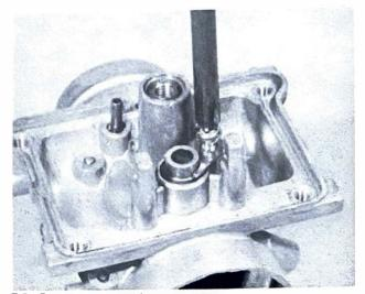
7.5a Remove screw and retainer plate ...
