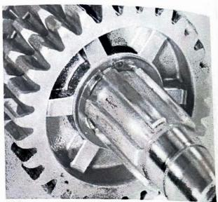
14.9d ... and secure with circlip
