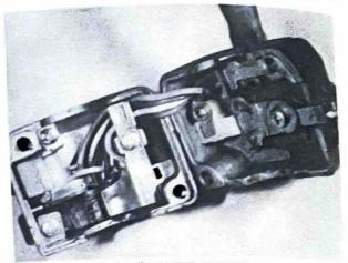
20.3 Switches can be dismantled for cleaning
