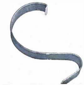
8.4a Home-made tool used to lock clutch centre (see photo 32.3f)
