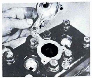
34.5d Fit the hose union, using a new gasket
