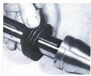
4.3c Slide off the rubber dust seal ...
