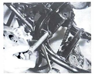
10.3c Remove nut and withdraw the pivot shaft ...
