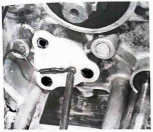
7.6a Release neutral switch lead from switch body
