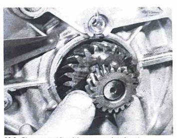
32.2a Place pump drive pinion over crankshaft end ...
