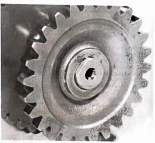
14.11d Fit the final thrust washer ...
