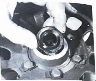
11.1f ... and seal to expose bearing
