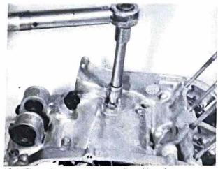
29.4a Fit crankcase upper bolts, noting wiring clips
