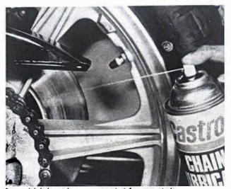
Aerosol lubricant is recommended for rear chain
