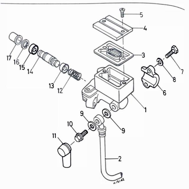
Fig. 6.2 Front brake master cylinder
