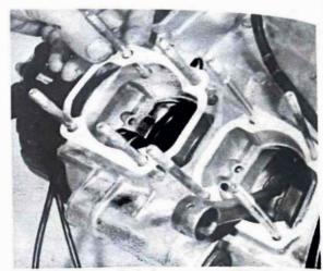
34.1a Place new cylinder base gaskets over holding studs
