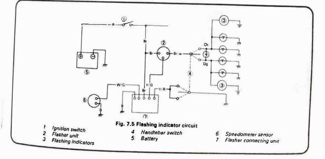
6 If the above tests reveal no obvious fault in the indicator circuits or the indicators will work only as a manually operated arrangement, the self cancelling system is inoperative and the unit will require renewal.
