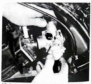
4.8b Slacken clips and disengage carburettors from stubs
