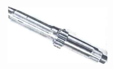
14.4a 1st gear pinion is integral with input shaft
