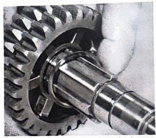
14.9c Slide 3rd gear pinion into place. Fit splined washer ...
