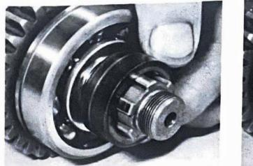
14.11g Bearing is followed by a steel spacer
