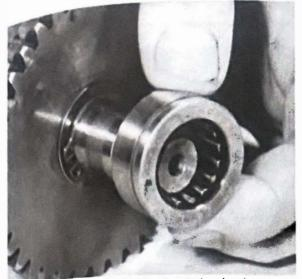
14.11a Fit the needle roller bearing to right-hand end ...
