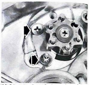
12.3b Release screws (arrowed) and remove drum retainer
