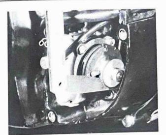
Check pump stroke adjustment with feeler gauges
