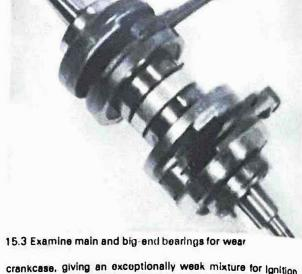
crankcase, giving an exceptionally weak mixture for Ignition, 3 It is unusual for the crankshaft seals to become damaged during normal service, but instances have occurred when particles of broken piston rings have fallen into the crankcases and lacerated the seals. A defect of this nature will immediately be obvious.
