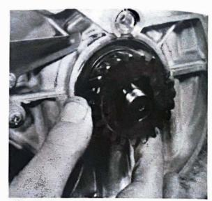
9.3d ... and the crankshaft pinion
