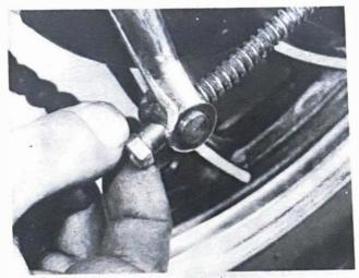
10.1 Remove the rear brake rod adjusting nut
