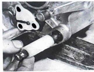
33.3 Connect neutral switch lead and fit gearchange sleeve
