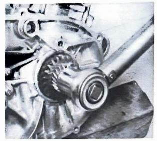
9.3a Lock crankshaft and slacken retaining nut
