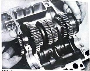
27.2a Lower output shaft into position ...
