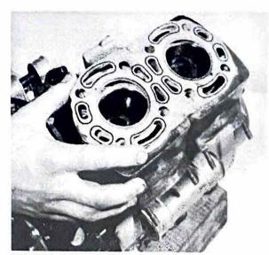
34.5a Place a new cylinder head gasket in position ...
