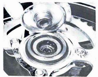
12.1a Remove flanged spacer ...
