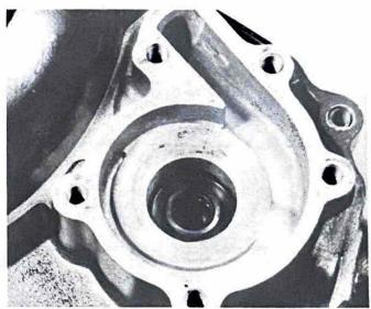
7.5b Ensure that seal locates properly in bore
