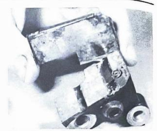
4.6d ... and shim and its retainer removed
