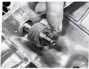
25.1b Gear is secured on shaft as shown
