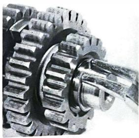
14.6d ... and retain with a circlip
