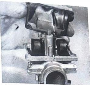
7.1b Remove float bowl taking care not to damage gasket
