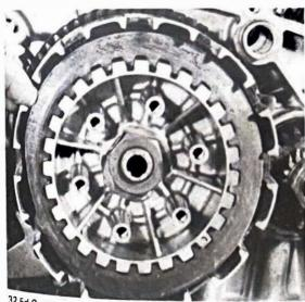
$^{32.5d}$  Cutaway of second plain plate is positioned  $60^\circ$  away from first
