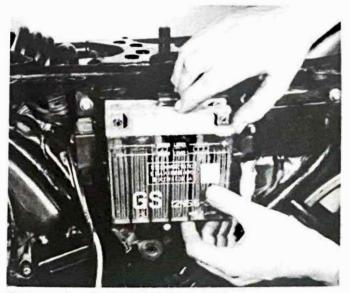
4.5d ... to allow the battery to be removed
