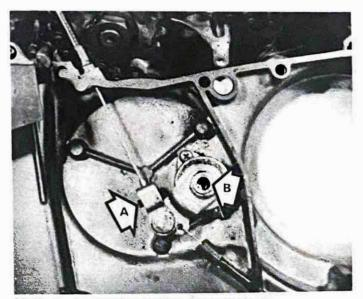
35.5a Bend over security tab A. Grease recess B
