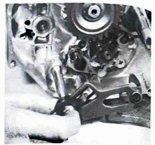
12.2 Displace gearchange shaft from crankcase
