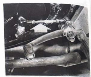
35.5e Mechanism can be adjusted to alter pedal height
