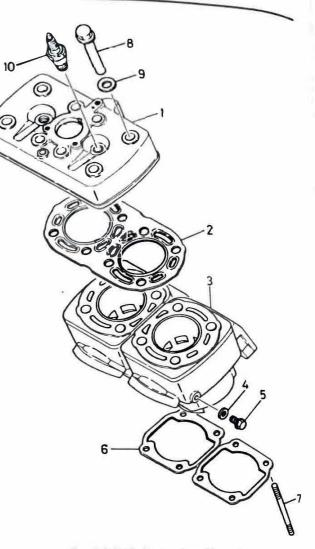
Fig. 1.1 Cylinder head and barrel
