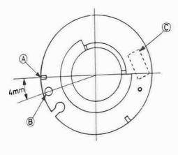
Oil pump pulley alignment marks
