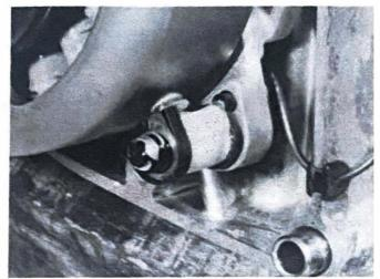
1.3 Pulser coil is mounted on extension of stator plate
