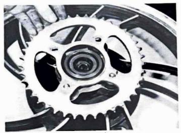
14.2d Sprocket can now be removed ...
