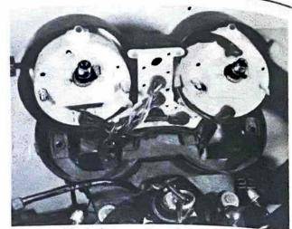
14.1b ... and lift the instrument panel away
