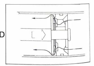
Fig. 5.4 Rear suspension unit operation
