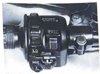
20.1b Left-hand handlebar switch unit
