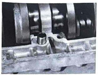
29.1 Apply jointing compound and fit locating dowels
