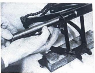
10.10 Inner pivot sleeve should be greased
