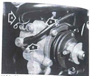
14.6 A: oil feed pipe from tank, B: oil delivery pipes
