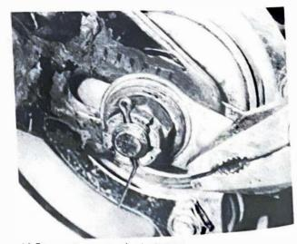
10.5b ... and rear wheel spindle nuts
