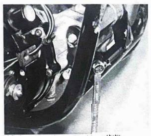
35.3a Assemble the front engine plates and bolts ...
