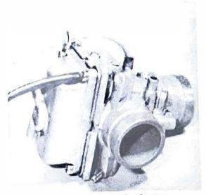
1a Float bowl is retained by four cross-head screws
