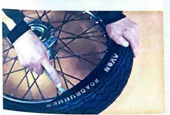
Use similar technique for second bead, finish at tyre valve position
