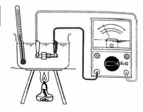
Fig. 7.7 Testing the cooling system temperature gauge sender
