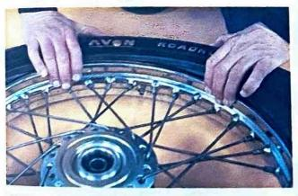
Lay tyre on rim and feed valve through hole in rim
