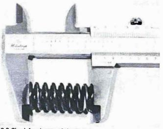
23.3 Check free length of clutch springs as shown
