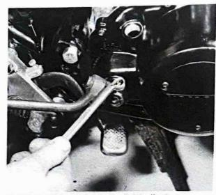
4.7a Remove kickstart pinch bolt and slide off splines
