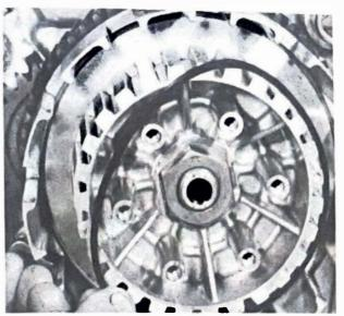
32.5a Commence clutch assembly with damper ring
