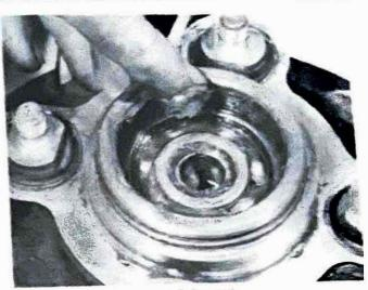
12.1h Grease bearing before fitting seal
