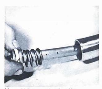
4.4b ... and shake damper rod out of stanchion
