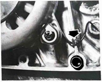
7.6b Note neutral switch lead grommet (arrowed)
