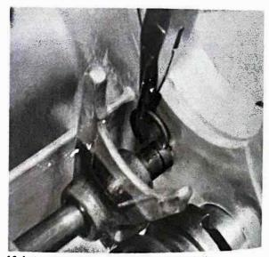
12.4a Use pointed-nose pliers to withdraw circlip ...
