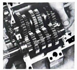
12.1 Remove gearbox shafts, noting position of half-rings
