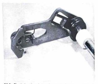
30.2a Check that the selector claw and springs are positioned as shown  $\ldots$
