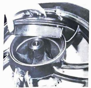
172 Litt brake backplate assembly out of hub
