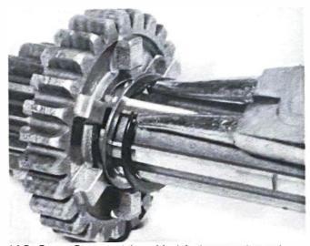
14.5a Secure 5th gear pinion with plain thrust washer and circlip
