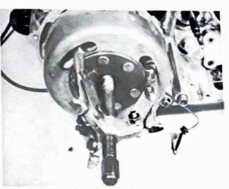
7.4 Assemble three-legged puller as shown
