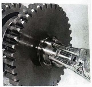
14.10b Fit 1st gear pinion with plain face outwards
