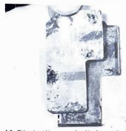
4.6e Shim should be removed and both parts cleaned
