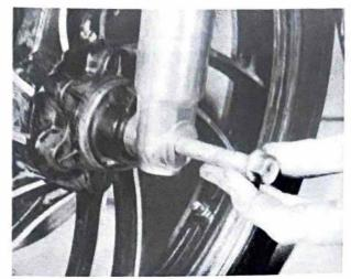
2.4b ... then withdraw spindle and remove wheel
