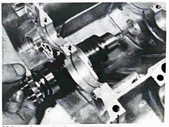
26.3a Lubricate and fit the gear selector drum
