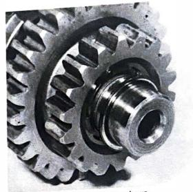
14.6c ... fit the plain thrust washer as shown ...
