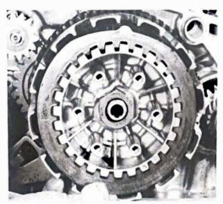
32.5c ... the first plain plate, noting cutaway portion
