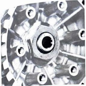
32.39 Do not omit to lock nut by bending up tab
