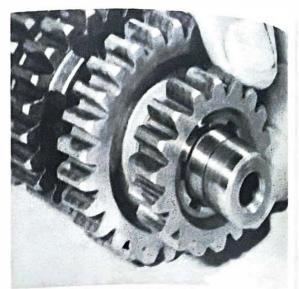
14.6b Slide 2nd gear pinion into position ....
