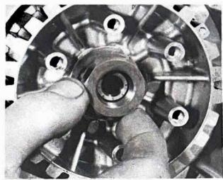
32.3e Fit tab washer and clutch centre nut
