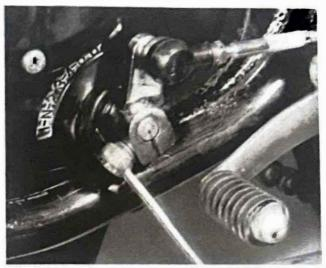
4.9a Release clamp bolt to free gearchange linkage
