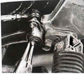
4.9b Pedal is retained by a circlip
