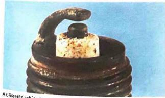
A blistered white insulator or melted electrode indicates overadvanced ignition timing or a malfunctioning cooling system. If correction does not prove effective, try a colder grade plug
