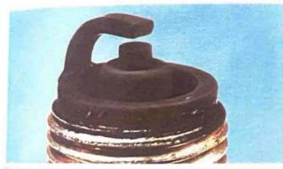
Black sooty deposits indicate an over-rich fuel/air mixture, or a malfunctioning ignition system. If no improvement is obtained, try one grade hotter plug
