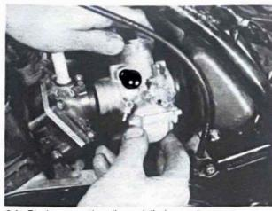
6.3a Slacken mounting clips and displace carburettors
