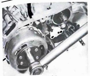
7.2 Lock crankshaft and slacken rotor bolt
