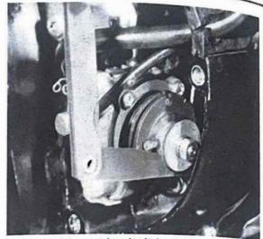
16.7 Measure pump stroke using feeler gauges
