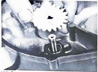
14.1b Remove pump pinion ...
