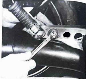
4.6b Silencer is secured by a single bolt
