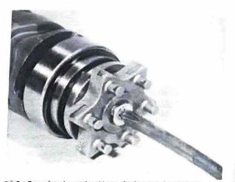
20.8s Camplate is retained by a single cross-head screw
