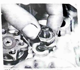
26.5b Fit the eccentric pin and retainer plate
