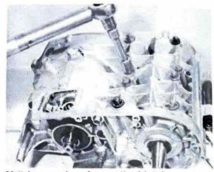
29.4b Lower crankcase is secured by eight bolts
