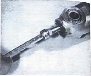
4.3b ... whilst bolt is unscrewed from fork leg
