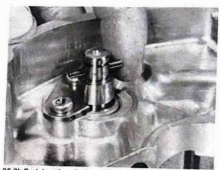
25.2b Push locating pin through hole in shaft ...
