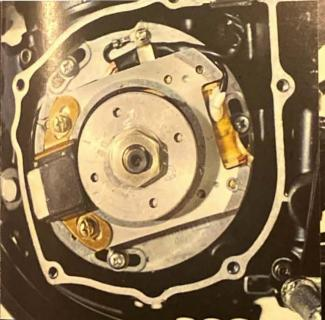
C.D.I. ignition system produces a hotter, more consistent spark at all engine speeds, and virtually eliminates spark plug fouling. It also eliminates all the problems that go along with conventional breaker points
