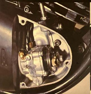
Autolube consistantly adjusts the flow of oil into the fuel mixture according to engine load and who want to save a little weight and premix, the unit is easily detachable
