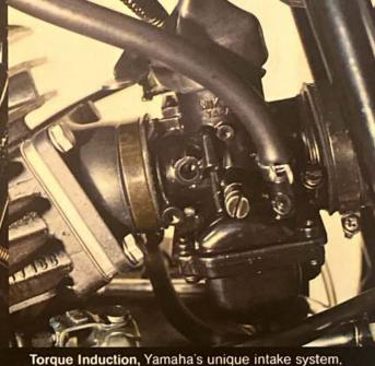
**Torque Induction,** Yamaha's unique intake system, utilizes a reed valve to feed the engine the exact amount of fuel and air it needs. The result is more horsepower, particularly at low rpm's.
