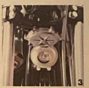
3. Hydraulic Disc damper for better handling on and off the road. It consists of an oil reservoir and a paddle in the steering column. When the handlebars are turned, the paddle works against the oil damping the left and right travel Ideal for dirt riding, since it pravents stones and ruts from radically deflecting the front wheel
