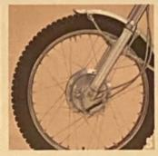
5 The extra-large front brake has positive, dependable stopping action Designed to be water and dustproof for safe stops in all conditions The rear stop lamp illuminates when front brake is operated for extra safety. The knobby tires assure positive traction anywhere so the machine responds instantly to acceleration or braking
