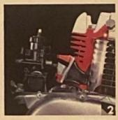
2. Exclusive Yamaha TORQUE INDUCTION<sup>®</sup> means better breathing and more horsepower at all rpm's Reliable stainless steel reed valve between the carb end cylinder opens on engine demand closes to prevent blow-back 7-port breathing means more power cooler running
