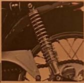
6 Double-spring, adjustable rear shock absorbers. One spring smoothsoutthe vibration caused by minor roughness in the road while the other spring cushions the larger shocks. The overall tension may be adjusted to any one of five positions according to the roughness of the road and the type of riding.
